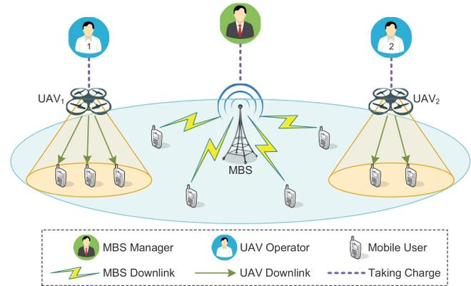
Fig. 1. The system model of UAV Assisted Offloading in Cellular Networks with 1 MBS manager and multiple UAV operators.
