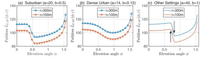
Fig. 9. (a) shows the pathloss in a typical suburban terrain, where parameters  $a = 5$ ,  $b = 0.2$ ,  $\eta_{LoS} = 0.1$ , and  $\eta_{NLoS} = 21$ . (b) shows the pathloss in a typical dense urban terrain, where parameters  $a = 14$ ,  $b = 0.12$ ,  $\eta_{LoS} = 1.6$ , and  $\eta_{NLoS} = 23$ . (c) shows a special case where there are more than one extremum points.
