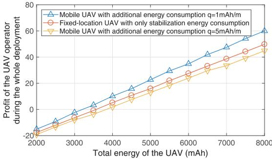
Fig. 8. The impact of the mobility and battery capacity of the UAV, with  $H = 200m$ ,  $M = 200$ ,  $\lambda_{BS} = 120$ .
