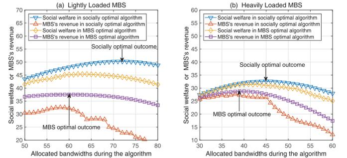
Fig. 5. The change of social welfare and MBS's revenue during the socially optimal algorithm and MBS optimal algorithm, where  $T = 10$ ,  $\{N_t\} = (1, 1, \dots, 1)$ ,  $\{\lambda_t\} = (1, 2, \dots, 10)$ ,  $M = 200$ , with  $\lambda_{BS} = 120$  for (a) and  $\lambda_{BS} = 160$  for (b).
