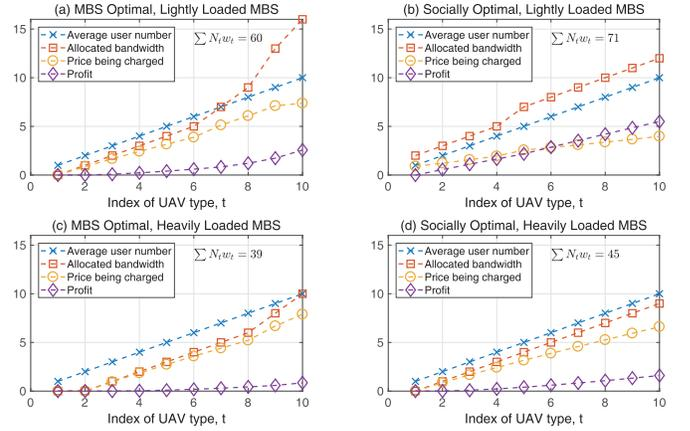
Fig. 4. The structure of the optimal contracts where  $T = 10$ ,  $\{N_t\} = (1, 1, \dots, 1)$ ,  $\{\lambda_t\} = (1, 2, \dots, 10)$ , and  $M = 200$ , with  $\lambda_{BS} = 120$  for (a) and (b), and  $\lambda_{BS} = 160$  for (c) and (d). In addition, (a) and (c) show MBS optimal contracts while (b) and (d) show socially optimal contracts.
